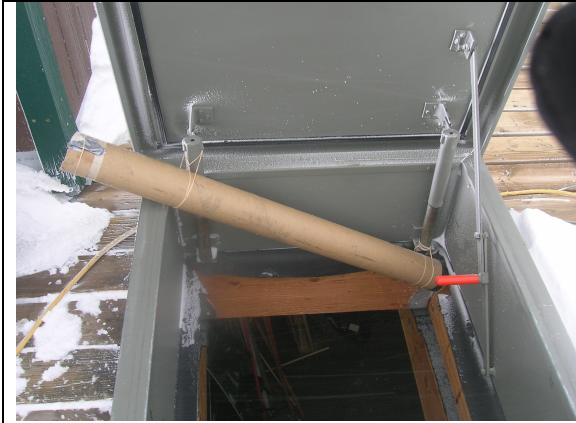
Figure 1c: Secondary Snow collection device.
