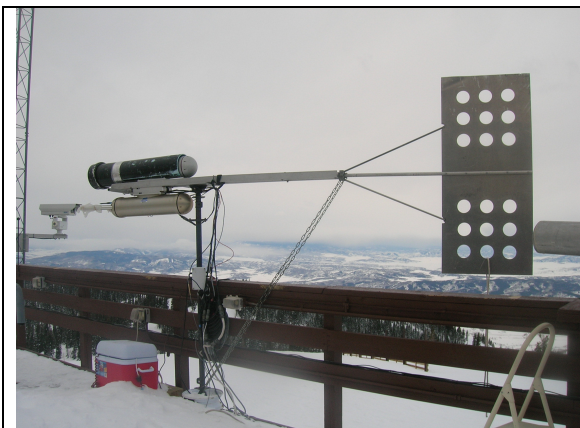
Figure 1a: Main Wind vane determining wind direction.
