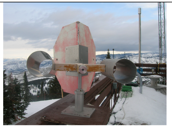
Figure 1b: Snow collection wind vane.
