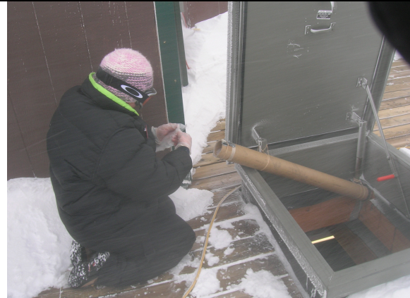
Figure 1d: Eagan attaching plastic snow collection bag to secondary Snow collection device.
