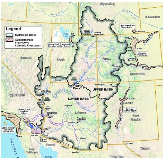
Figure 7.3. Map of the Colorado River compact among the states of Colorado (3.9 million acre-feet), Wyoming (1.0), Utah (1.0), Arizona (2.8), New Mexico (0.9), Nevada (0.3), and California (4.4). It is based on an assumed river flow of 18 million acre-feet.
