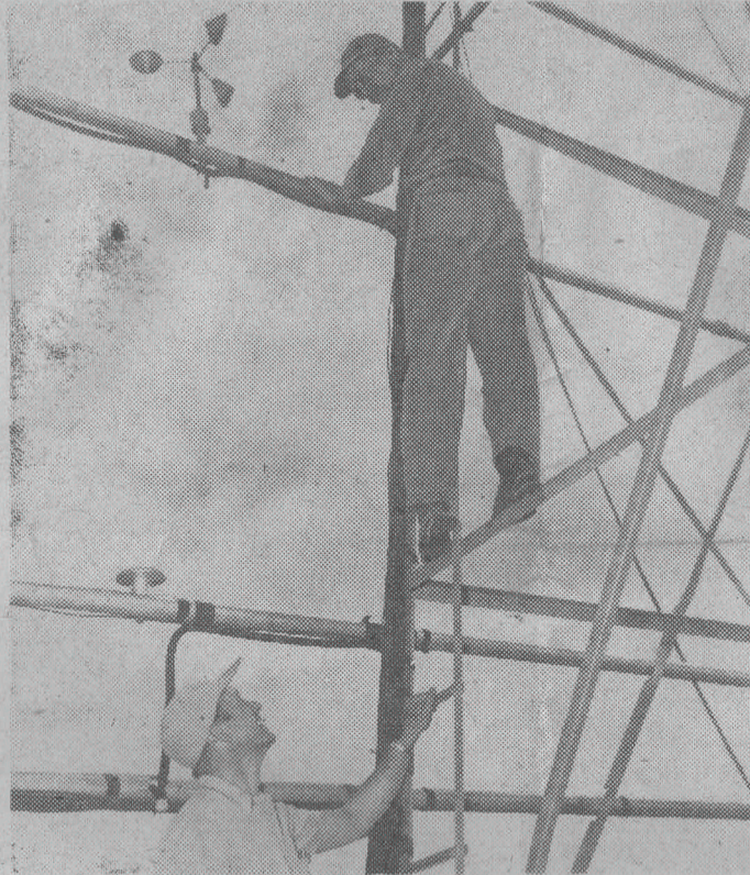
Dr. Harrison Cramer (on tower) and Dr. Frank Record of Massachusetts Institute of Technology inspect wind measuring instruments at the O'Neill test site. They are measuring rapid changes in wind speed at low levels.
